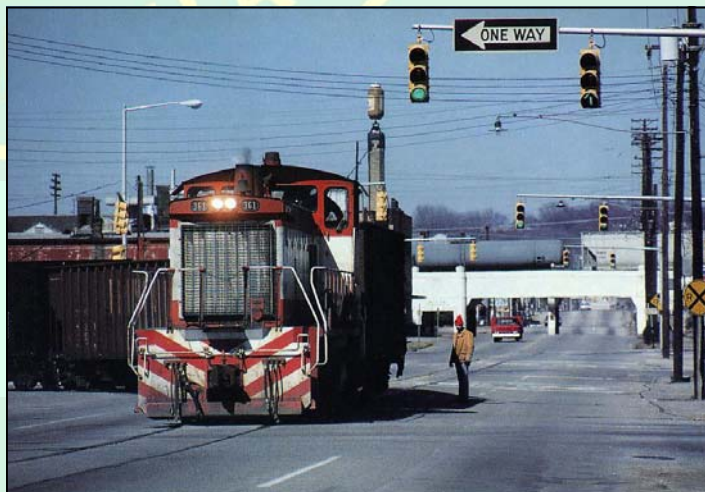
Switching a cut on a sharply curved industrial spur while obeying traffic signals along 14th Street South
