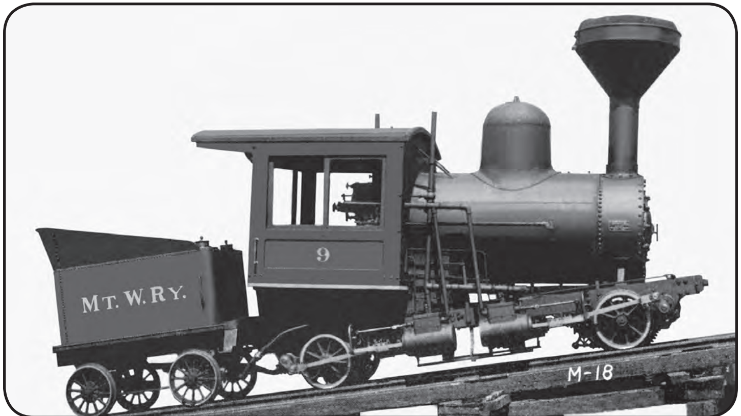
Rack Loco - Mt. Washington cog engine No. 9 was built in 1906 by Manchester (NH) Locomotive Works, and served until arrival of diesels. It used 130 psi boiler pressure, weighed 26,700 lbs, and had a reactive effort of 7000 lbs.
