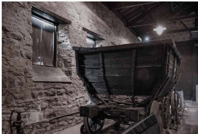
Figure 7. Early 1800s wooden rail cauldron wagon from Northeast England. Photo by Ken Boyd.
