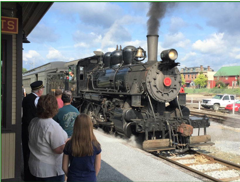
Engine No. 11 arriving at the Hollidaysburg depot. Built by Alco in 1920 and intended for export but never left the country. We restored it to operation in 2015. Since this photo was made, it has been converted from coal to oil firing. (Photo by Alan Maples)
