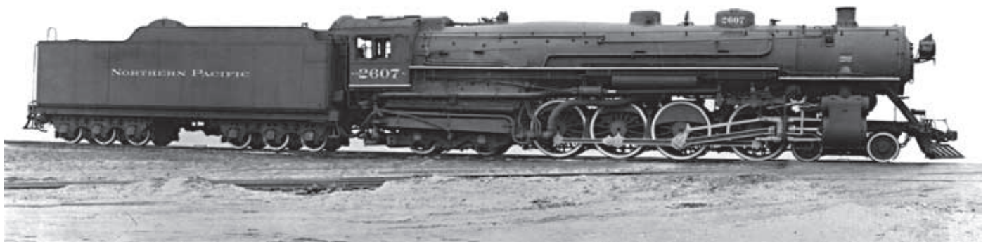
Northern Pacific 4-8-4 No. 2607, built by American Locomotive Company in 1927, part of Order No. S-1559 for locomotives 2600 through 2611. Photo by American Locomotive Works, R&LHS Frank M. Swengel Collection.
