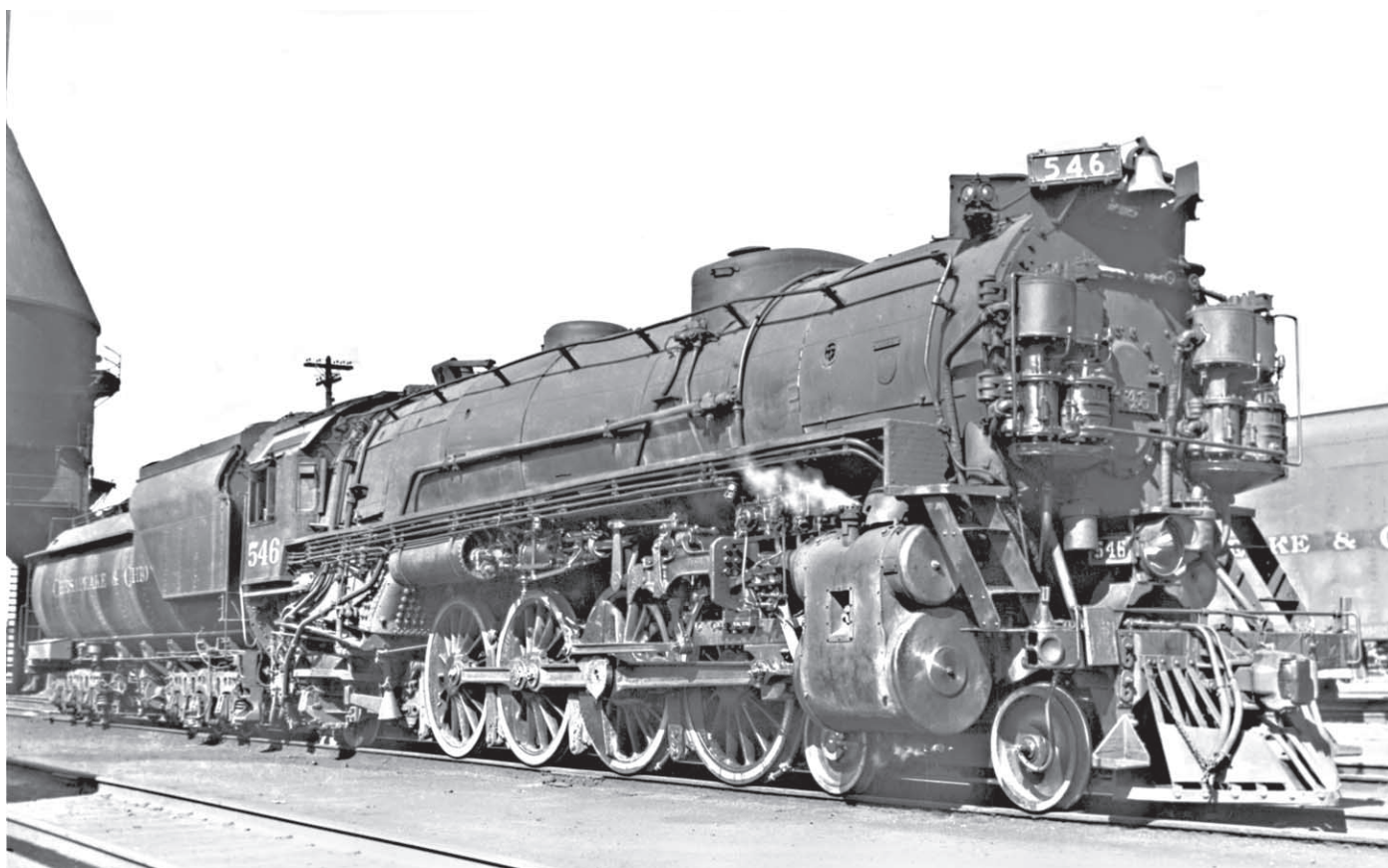
With low-water alarm, mechanical lubricator, multiple-bearing crossheads, modified cab, “flying pumps,” sloping pilots, and 16,000 gallon Vanderbilt tender, C&O #546 hardly looks the same. Built originally by Baldwin in 1919, she is at Richmond, Virginia, March, 1948. H. K. Vollrath collection.
