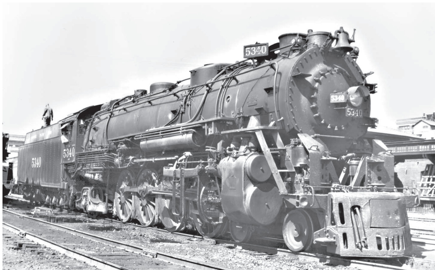
Missouri Pacific #5340, shown at Texarkana, Kansas, September, 1949, illustrates the evolution of the USRA light and heavy Mountain types. Built by Schenectady in 1930, this handsome passenger engine can be traced back to USRA 4-8-2s nos. 5301-5307, Richmond, 1919. H. K. Vollrath collection.
